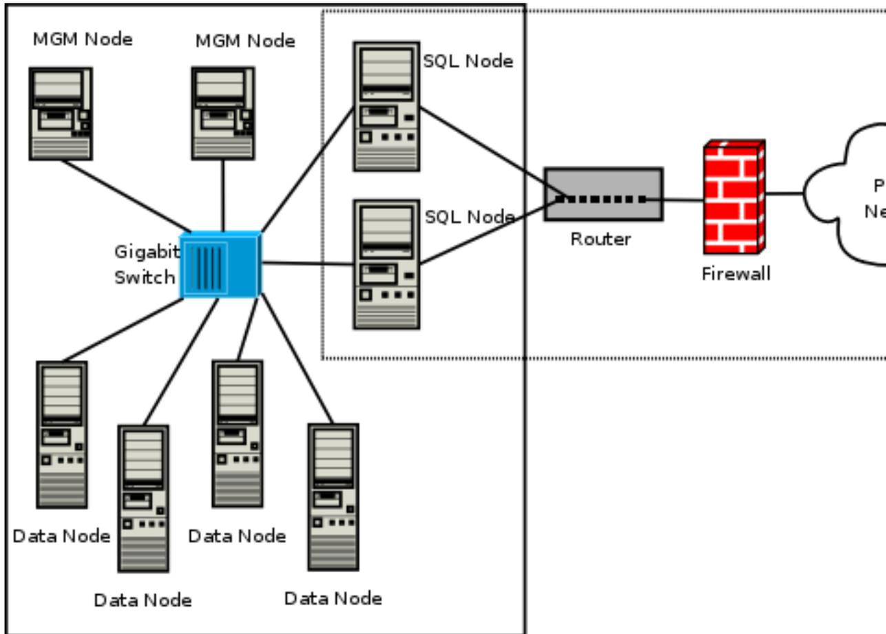
This setup has two networks, one private (solid box) for the Cluster management servers and data nodes, and one public (dotted box) where the SQL nodes reside. (We show the management and data nodes connected using a gigabit switch since this provides the best performance.) Both networks are protected from the outside by a hardware firewall, sometimes also known as a *network-based firewall*.
