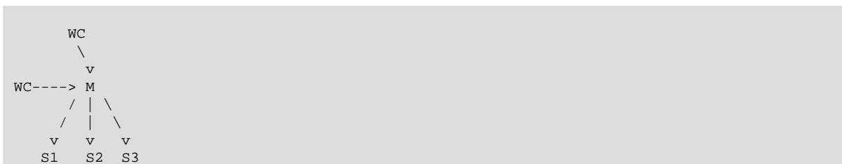
In this diagram, **M** means the master, **S** the slaves, **WC** the clients issuing database writes and reads; clients that issue only database reads are not represented, because they need not switch. **S1**, **S2**,
