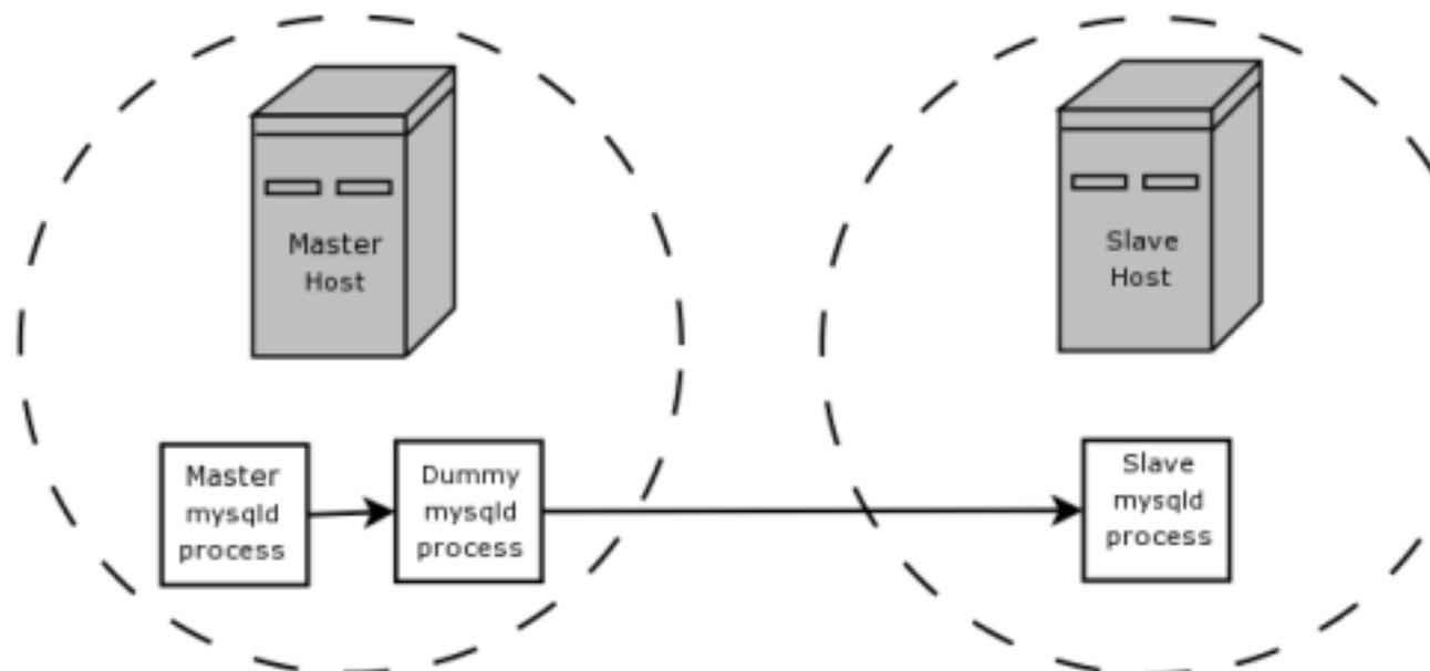
The master writes to its binary log. The “dummy” `mysqld` process acts as a slave, applying the desired combination of `replicate-do-*` and `replicate-ignore-*` rules, and writes a new, filtered binary log of its own. (See [Section 14.8, “Replication and Binary Logging Options and Variables”](#).) This filtered log is provided to the slave.
