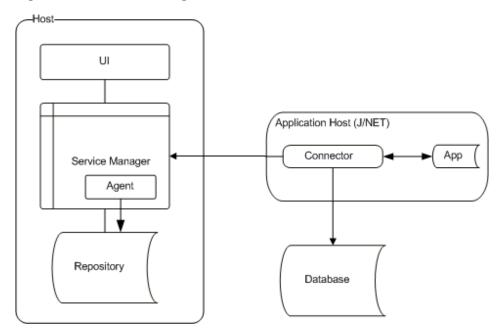
Figure 12.2 Connector Plugin Architecture
