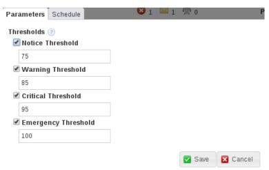
The values shown are taken from the Availability Advisor, **Maximum Connection Limit Nearing or Reached**. The values define the percentage of maximum connections at which an event is logged. For example:
