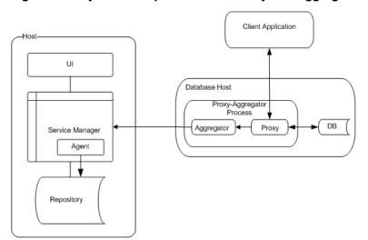
Figure 11.1 MySQL Enterprise Monitor Proxy and Aggregator Architecture
