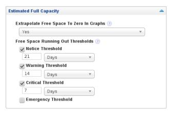
The **Estimated Full Capacity** section monitors and graphs the time remaining to full capacity based on existing load.
