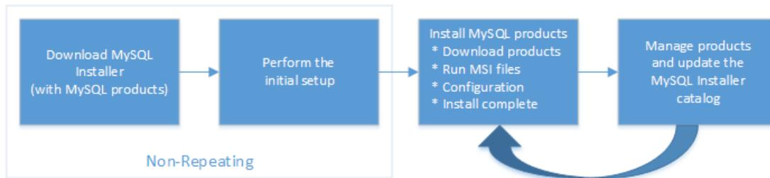
MySQL Installer extracts configuration files (described later) to the hard drive of the host during the initial setup. Although MySQL Installer is a 32-bit application, it can install both 32-bit and 64-bit binaries.
